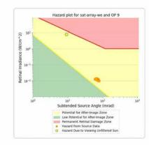
PV array is expected to produce the following glare for this receptor: • 0 minutes of "green" glare with low potential to cause temporary after-image.
