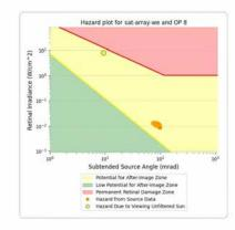
PV array is expected to produce the following glare for this receptor: • 0 minutes of "green" glare with low potential to cause temporary after-image. • 1,512 minutes of "yellow" glare with potential to cause temporary after-image.
