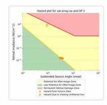
PV array is expected to produce the following glare for this receptor: • 4 minutes of "green" glare with low potential to cause temporary after-image. • 152 minutes of "yellow" glare with potential to cause temporary after-image.
