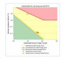
PV array is expected to produce the following glare for this receptor: • 0 minutes of "green" glare with low potential to cause temporary after-image. • 826 minutes of "yellow" glare with potential to cause temporary after-image.
