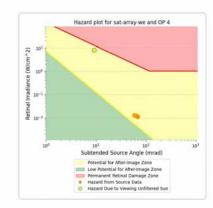
PV array is expected to produce the following glare for this receptor: • 0 minutes of "green" glare with low potential to cause temporary after-image. • 1,212 minutes of "yellow" glare with potential to cause temporary after-image.
