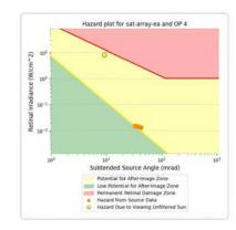
PV array is expected to produce the following glare for this receptor: • 0 minutes of "green" glare with low potential to cause temporary after-image. • 257 minutes of "yellow" glare with potential to cause temporary after-image.
