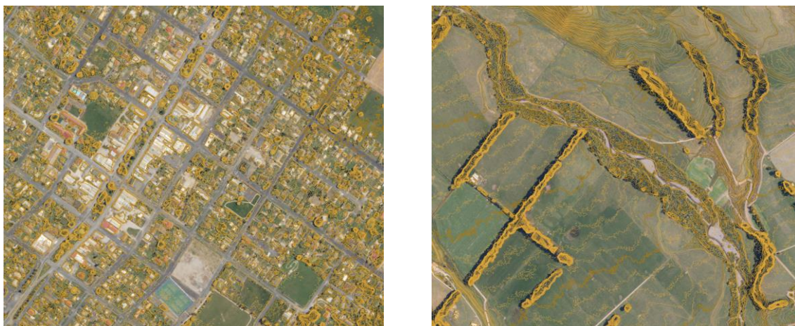
Figure 3.4: Examples of areas where buildings and trees have not been removed from the elevation data and therefore have distorted the contours created for this assessment at 1:5,000 scale. Left: buildings in Pahiataua; Right: trees and vegetation along streams and in farmland to the north-west of Dannevirke.
