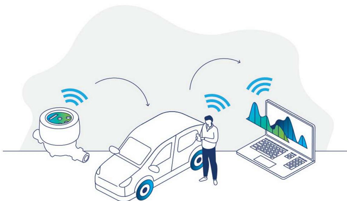
Figure 4-2: Schematic of an Automated Meter Reading (AMR) System as Applied to Water Metering. Source: https://arad.co.il/amr-ami/drive-by-walk-by/ .
